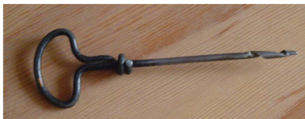
Fig. 2 A gimlet, such as the one pictured was used during the ‘subcutaneous’ osteotomy technique by Prof. Pancoast to create multiple femoral perforations at the osteotomy site (image from Wikipedia)
